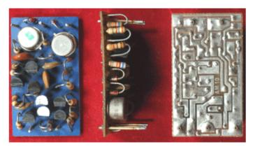
The garAM10BC is a 2520 pinout modern version. It uses 5% Murata Caps and 1% metal film resistors. The Transistors are all current production BC550C/BC560C TO92 small signal transistors and BD139-16/BD140-16 otuput transistors.
